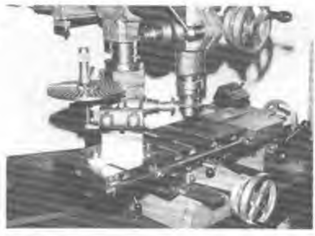
Fig. 81 Ready to cut a bevel gear on a vertical milling machine. Note angle of dividing head.
